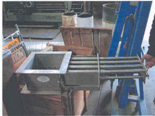
Figure 3.8 Magnetic separator supplied by SACBH and used to trial the separation of meghemite from canola seed.
