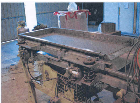
Figure 3.1 Screening deck at AMRDC used to trial the separation of meghemite from canola seed
