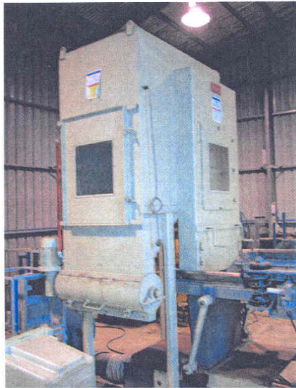
Figure 3.6 Air separation unit at AMRDC used to trial the separation of meghemite from canola.
