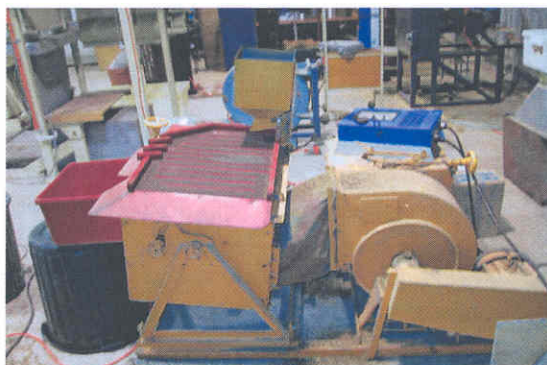
Figure 3.3 Specific gravity separation table at AMRDC used to trial the separation of meghemite from canola.
